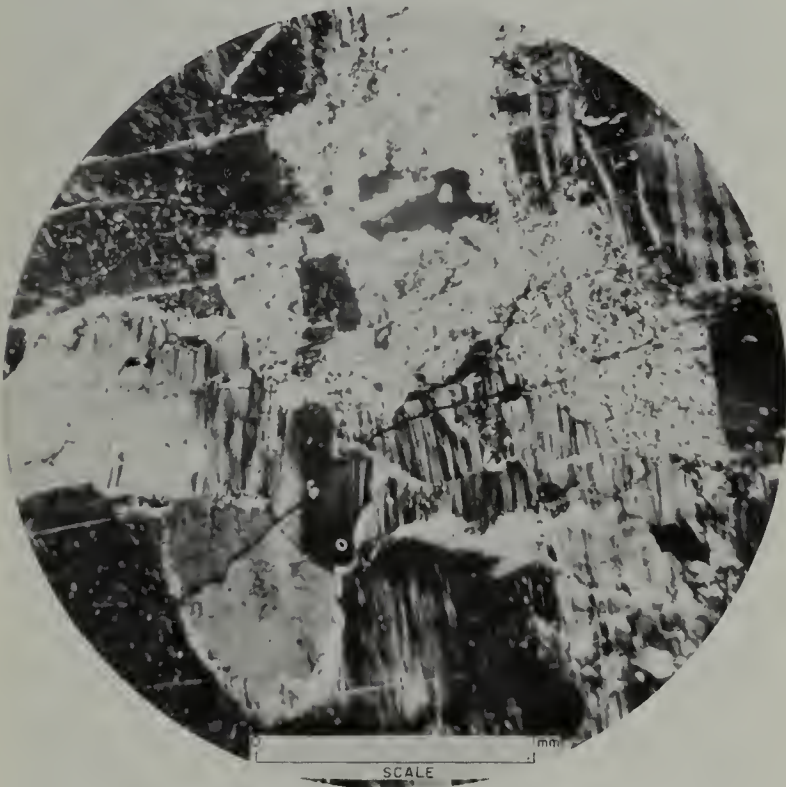
Photo 3. Biotite augen gneiss, showing replacement of sericitized plagioclase (light-colored in center) by microcline (dark, with quadrille structure, surrounding plagioclase). In upper left quadrant microcline shows embayment relation toward plagioclase. Crossed nicols.
